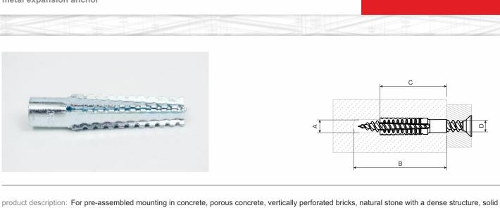
brickwork blocks, solid sand- lime bricks. The external teeth expand in the building material, thus ensuring a high load-bearing capacity. Thread must be screwed in at least min. to the full length of the anchor. The length of the anchor is calculated: length of the anchor + bolt diameter + thickness of the
